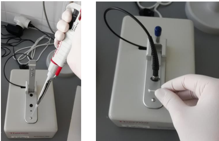
Fig. 8: Sample transfer into the NanoDrop machine
